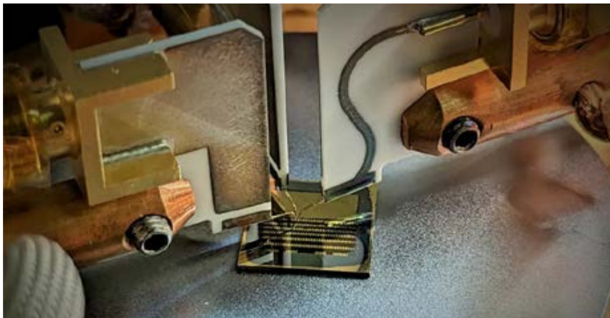
The millimetre-sized chip on which the transistors are located. Photo: Anton Persson
